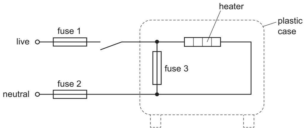
Which of the fuses are correctly placed?
